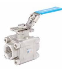
3-piece 2000 CWP carbon or stainless steel ball valve, API 607 fire tested (standard), ISO 5211 direct mount actuator pad, locking handle, tongue & groove body seal, spring loaded packing, in-line maintainable
