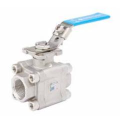
Characterized control valve with V-port ball, ISO 5211 actuator mounting pad, locking lever handle, Graphoil packing, API 607, 5th Edition fire tested
