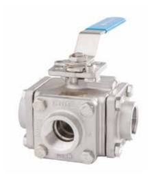
3-way L or T port ball valve, 4 seated, bolted-on end caps, anti-static stem, ISO 5211 actuator mounting pad, locking handle
